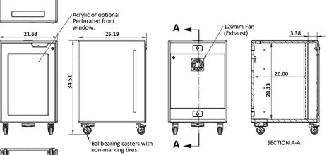
The mobile rack model **REX16** includes front and rear 16U rack rails for equipment up to 20" deep, framed front door with a tinted acrylic window and heavy duty casters for easy maneuverability.
